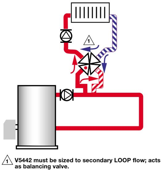
Fig. 8 Injection configuration.
