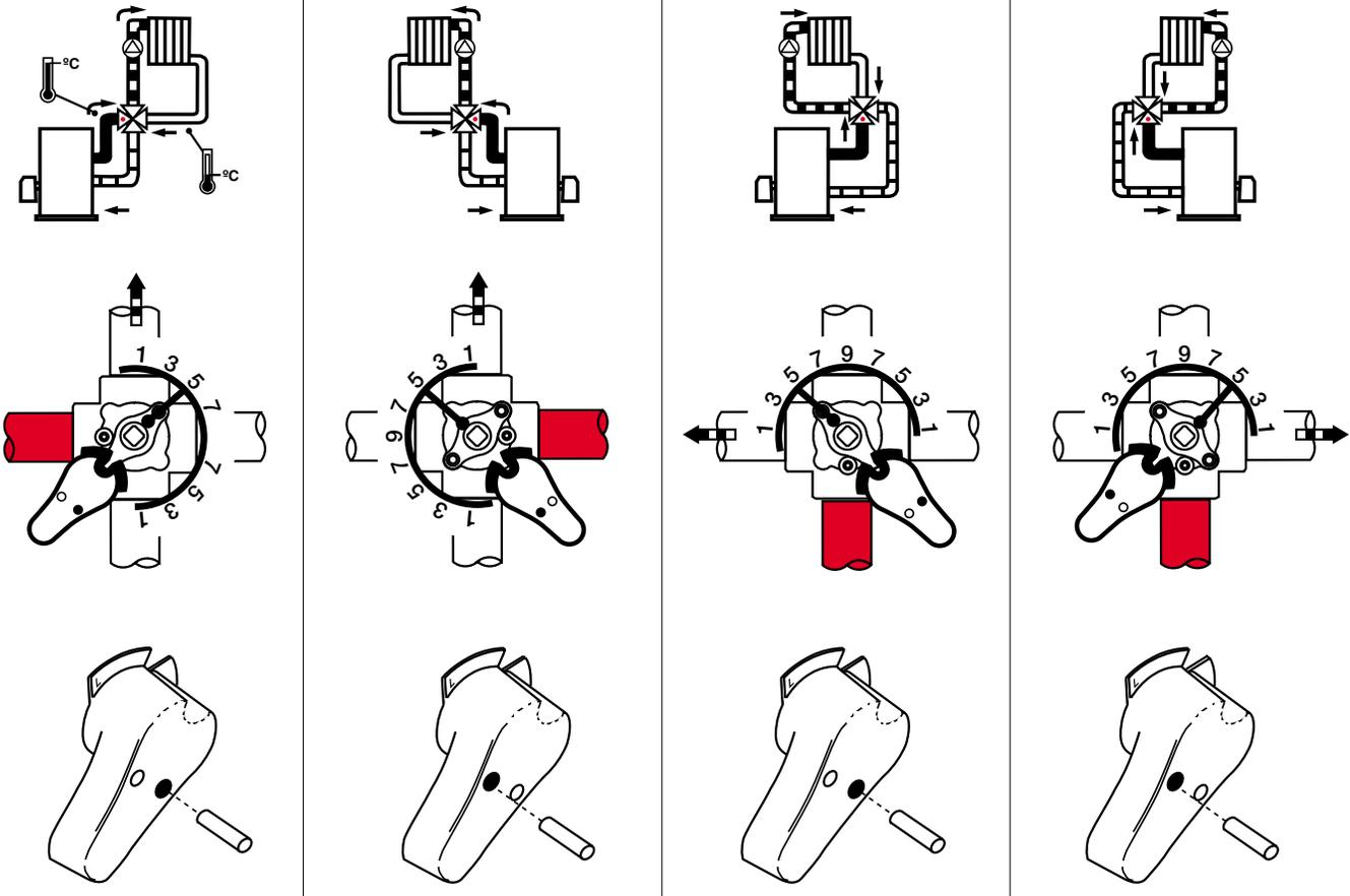
Fig. 5 Single mixing valve installation
